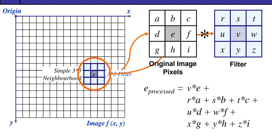
The above is repeated for every pixel in the original image to generate the filtered image
